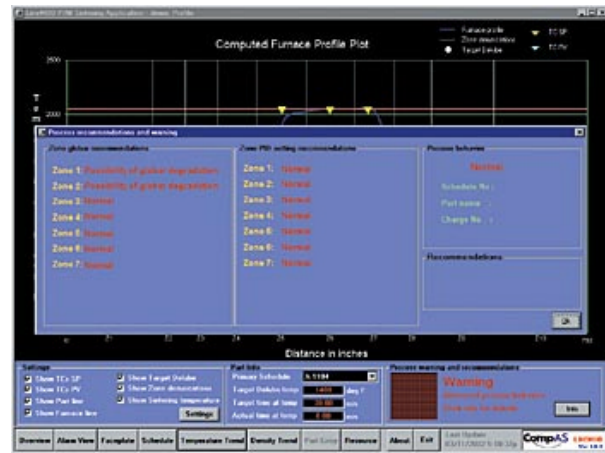
Fig 4 Imminent furnace heating-element failure is predictable using control software diagnostics
