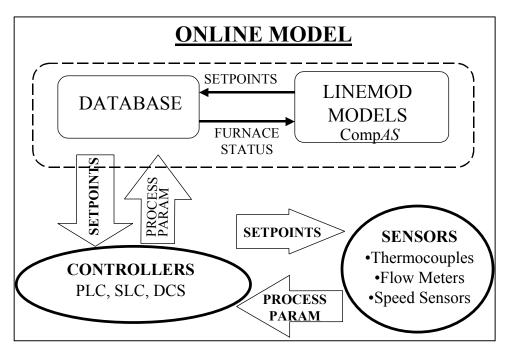
Following are the major elements (subsystems) of the core software. These elements work together to facilitate the control and provide operational insight into the process.
