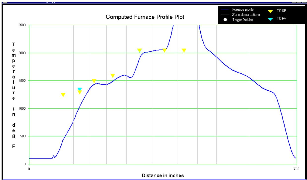
Figure 7: Thermocouple failure in sintering zone # 3.
