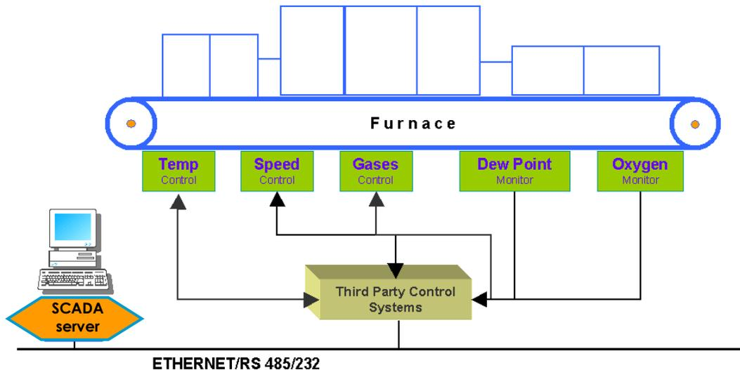
Figure 2. Schematic of communication for the SCADA system.
