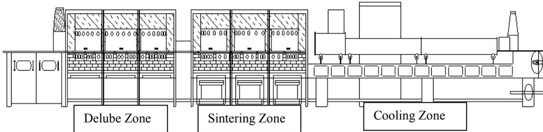
Figure 3: Furnace-schematic
